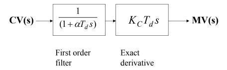
The first term is a filter that reduces the "noise" in the signal. The parameter alpha  $(\alpha)$  is small, usually about 0.10, so that the filter does not unduly slow the response of the derivative. The second term is the exact derivative which acts on the signal after filtering.
