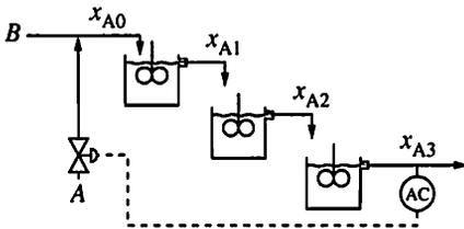
The reader should recall the likely accuracy in the dynamic model when tuning a PID controller. The gain, time constant, and dead time from empirical identification have significant errors (20 percent is not uncommon); therefore, precise values from the correlations are not required, because small errors in reading the plot are insignificant when compared with the modelling errors. The use of the correlations is demonstrated in the following examples.
