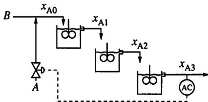
reasonable range, is certainly not too large, and should not cause oscillatory behavior. The conclusion is that the integral time is too short. The transient response with double the integral time is that shown in Figure 9.12, confirming that reasonably good control performance can be achieved by changing only the integral time.
